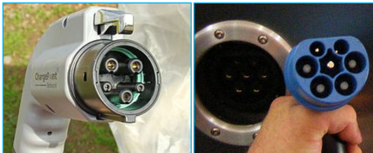
Figure 7.4: Type 1 and Type 2 EV Charger Plugs
